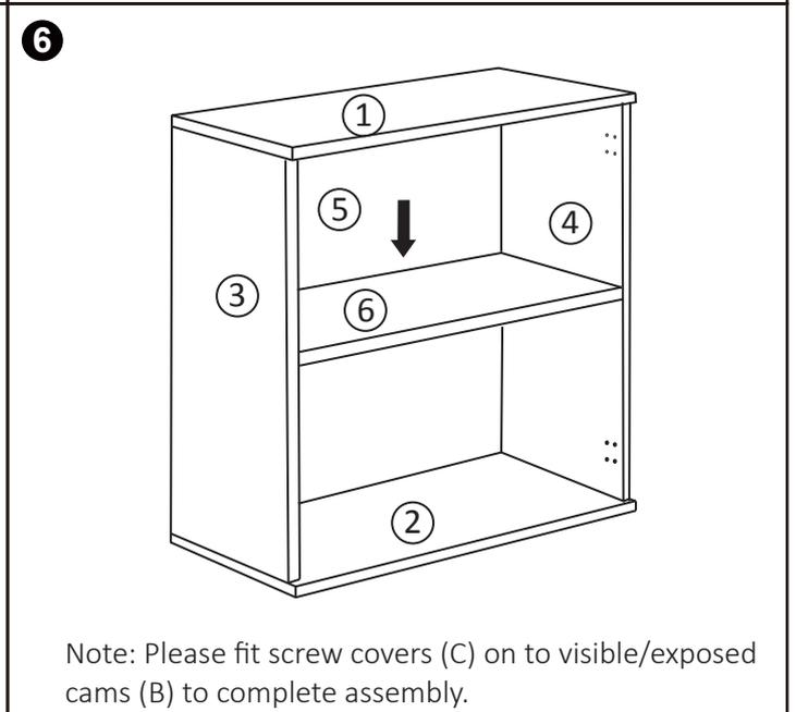
**Only tighten the screws by hand with provided allen key.
