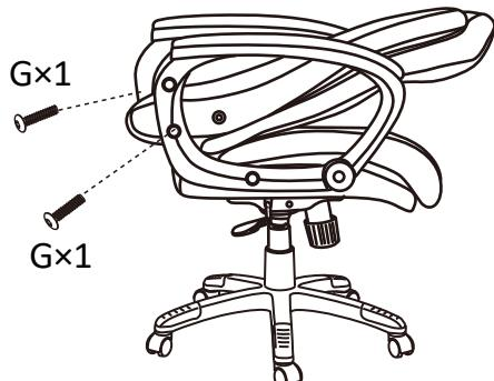
**6** When all the bolts are in position, fully tighten
